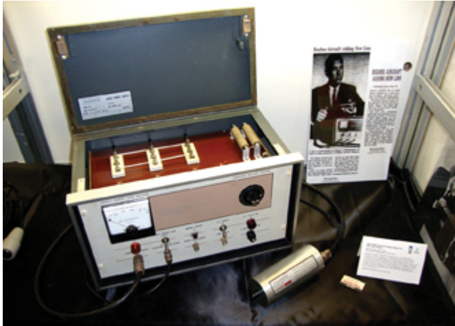
Figure 2. Built in 1962, the Model 200 ruby laser system was the first commercial laser product built by Hughes Aircraft Company. It was part of the Laserfest exhibit at Photonics West in 2010.
