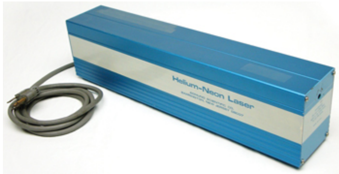
Figure 10. This 1969 Edmund Scientific model 79006 HeNe laser was intended for educational applications and features an easily removable plasma tube for easy experimentation.
