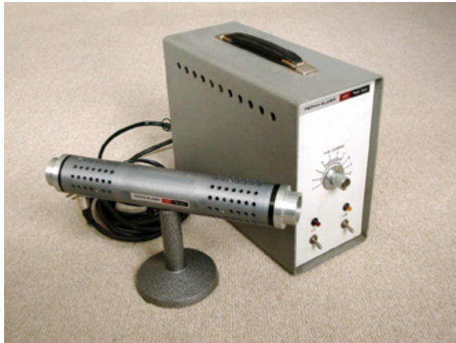
Figure 5. The 1966 PerkinElmer Model 5200 HeNe laser system, originally offered in 1963, was also used in the company's laser Raman spectrometer, first offered in July 1964. A very " '60s looking" laser!
