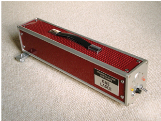
Figure 8. The 1967 Scientifica & Cook Model B17/S HeNe laser, an early British laser from the “Summer of Love,” shows a classic ’60s design.
