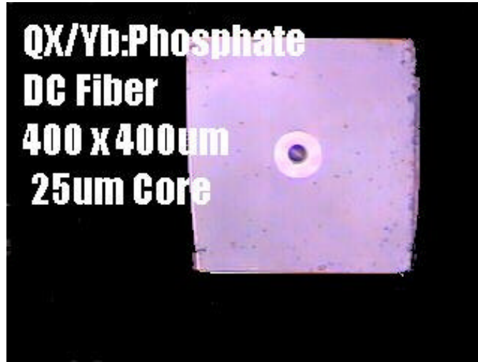
Figure 5 Cross-section view of QX/Yb DC LMA fiber
