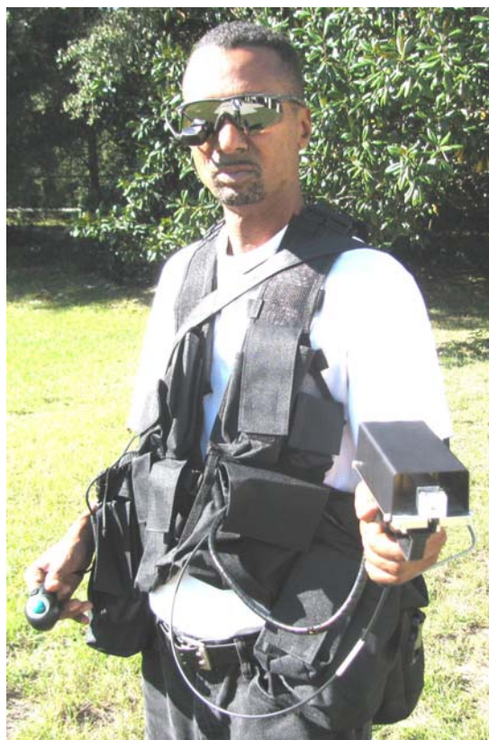
Fig. 13 - Wearable LIBS system components assembled on engineer
