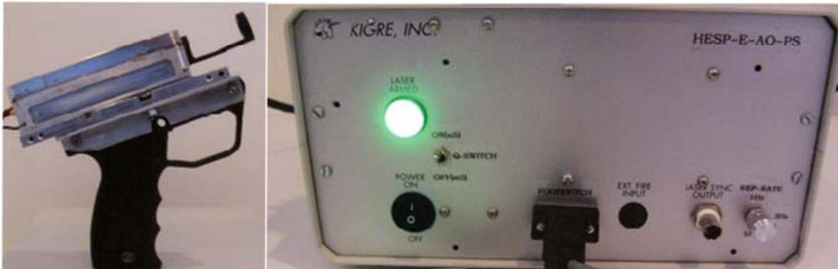
Figure 6. AO-1010 laser head (mounted on paintball gun grip) and laboratory power supply front panel [28,29,30].
